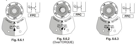
When torque on valve shaft exceeds the value set, e.g. running to close, shaft T turns to the right (Pointing to FPC), at the same time central SHAFT releases (See figures 8.6.1 and 8.6.2). FPC microswitch is tripped. Automatically, or when actuator starts running to opposite direction, mechanism returns or resets. Notice that central SHAFT latches again. (Figure 8.6.3)
