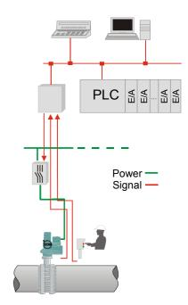
The electric actuator is a device designed to be coupled to a general purpose industrial valve, to carry out its movement. The movement is stopped by limit switching or by torque (thrust) switching. Other applications should be consulted CENTORK before. CENTORK is not liable for any possible damages resulting from use in other than designated applications. Such risk lies entirely on the user.
