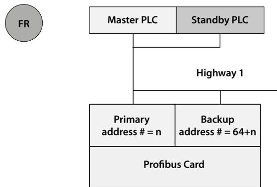
Fig. 21: Flying Redundancy – One highway redundancy
