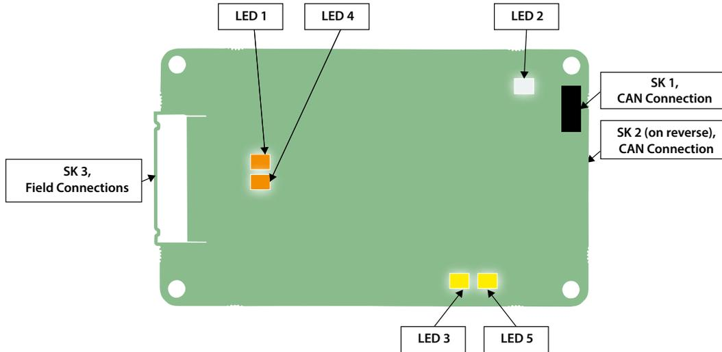
Fig. 22: Dual Channel Profibus card LED positions
