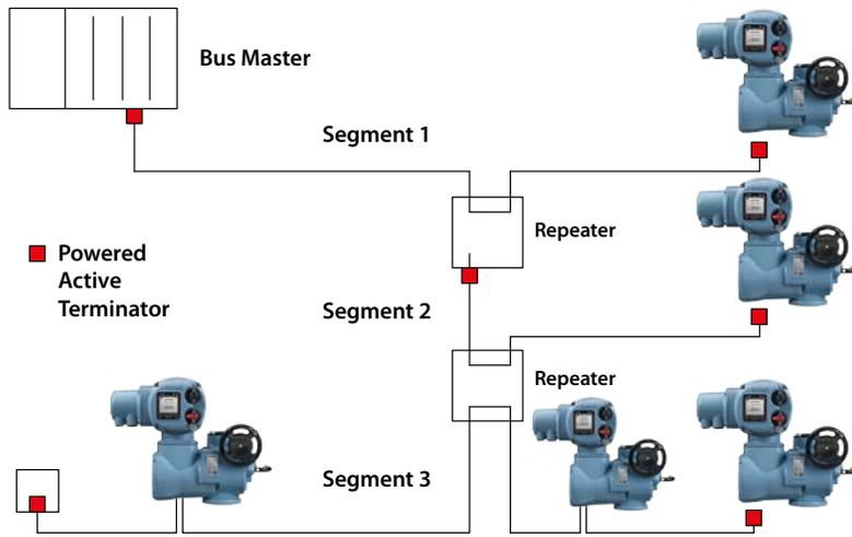
Fig. 6: Profibus Single Channel Data Highway Topology
