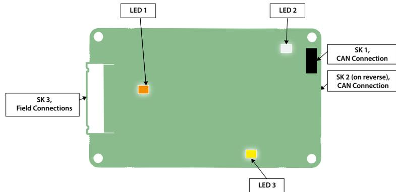
Fig. 19: Single Channel Profibus card LED positions
