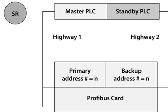
Fig. 20: System Redundancy – Two highway redundancy
