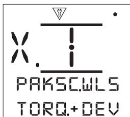
**Torque Update Time [TORQ.+DEV.]:** - Set for the amount of change in actuator measured torque that has to occur before torque data is reported to the master station. During valve travel, torque reporting will be made each time the torque changes by more than this setting. If torque data is not being used then the deviation should be set to disabled. Range 0% (Disabled) to 20%.
