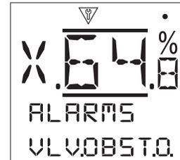
**Valve Obstructed [VLV.OBST.]:** - Displays the Valve Obstruction alarm status. When active, this alarm indicates that the valve is obstructed or has reached the torque limit set. Check that the valve is free of any obstruction and is operating correctly.
