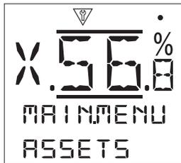
Asset management is an increasingly desirable requirement in process industries and can be used to manage valve asset performance, availability and maintenance schedules. Information regarding the process, valve and actuator can be stored in the Centronik module. In addition to this, the installation and commissioning dates along with the service history of the actuator can be recorded. Asset management alarms can also be set to indicate possible maintenance required.
