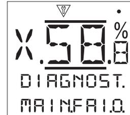
**Mains Fail [MAIN.FAI.]:** - Displays Power Supply failure status. When active, this status indicates a power supply failure has occurred. If the backlight is still present it is likely that the third phase has been lost. Check all incoming phases.
