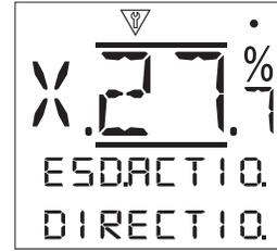
**Direction [DIRECTIO.]:** - Set the desired ESD movement direction.
