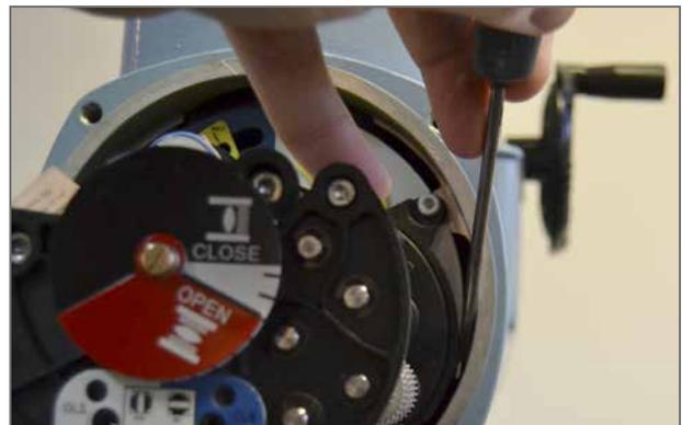
**N/C CLS** – Normally Closed (break when active) Close Limit contact for motor control
