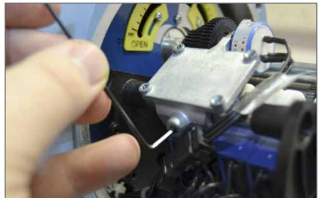
\*Potentiometer terminals may not be accessible if the AID CPT option is also fitted. In this instance it is important to ensure the POT does not slip throughout full valve travel. Current should change through 4-20 mA however tuning may be required. Refer to the next page for tuning instructions.
