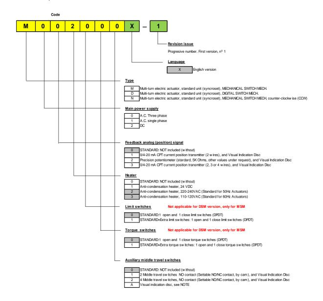
CK range actuators have an assigned wiring diagram and terminal plan for the specific build of the subject actuator. These are incorporated into one document that details the electrical connections and terminal allocations within the unit. Each document has an assigned code that will be required for actuator commissioning support.
