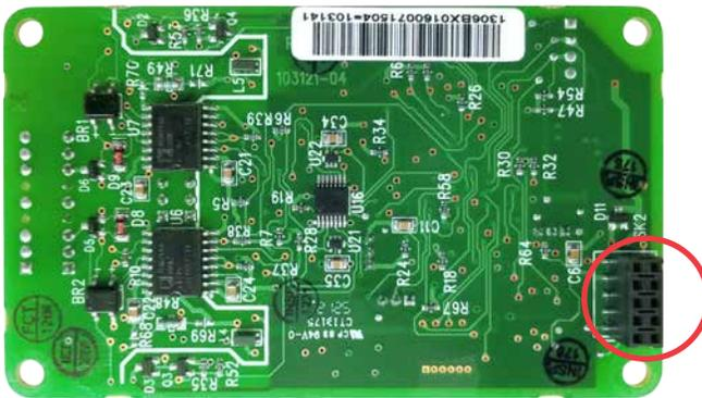
Control board connection. SK2 connector fitted on underside of MFU.
