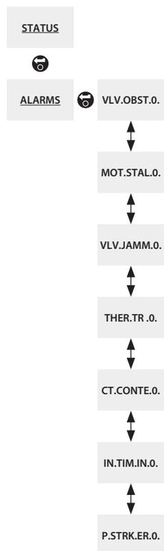
The above menu map should be used as a navigation prompt to improve configuration efficiency. An underlined text string indicates a menu. A standard text string indicates a setting.
