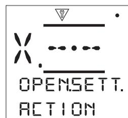
**Action [ACTION]:** - Specify the valve opening action – Seat Limit or Seat Torque.
