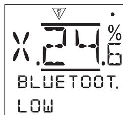
**Low: Always [LOW]** – The actuator is available at all times for *Bluetooth* communication using a PC running Accent Software. This setting provides convenient connection when Accent is used. Communication with the *Bluetooth* Setting Tool is available.
