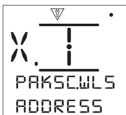
**Address [ADDRESS]:** - The Pakscan Field Control Unit option must be allocated a unique wireless loop node address. Changes made to the address will take effect immediately. The range of address is 1 to 300.
