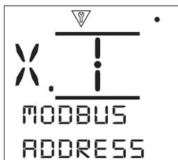
**Address [ADDRESS]:** - The Modbus option must be allocated a unique address to which it is attached. Changes made to the address will take effect immediately. The range of address is 1 – 247.
