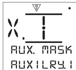
**Auxiliary 1 [AUXILRY.1]:** - Refer to Auxiliary input setup table below.
