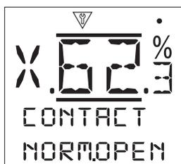
**S Contact [CONTACT]:** - Each relay contact output can be configured as normally open (make on condition) or normally closed (break on condition) to suit either type of field wiring.
