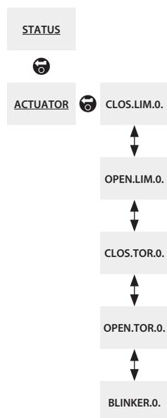
The above menu map should be used as a navigation prompt to improve configuration efficiency. An underlined text string indicates a menu. A standard text string indicates a setting.
