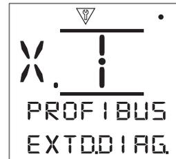
**Extended Diagnostics [EXTD.DIAG.]:** - Used for dual channel Profibus option (redundant) only. Refer to wiring diagram. The slave redundancy specification from the PNO describes extended diagnostics that are available in the redundant card. These messages describe, for example, the state of the backup channel. Diagnostics messages can be turned on and off depending on the capabilities of the PLC to which the module is connected.
