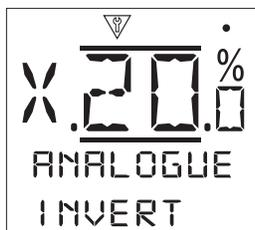
**Invert [INVERT]:** - Specify whether the output 4-20mA signal increases or decreases whilst the actuator is moving open.
