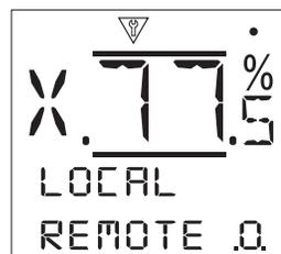
**Remote [REMOTE]:** - Displays the current Remote signal status. When active, this indicates the local controls have been set to remote and a remote mode signal is being received.
