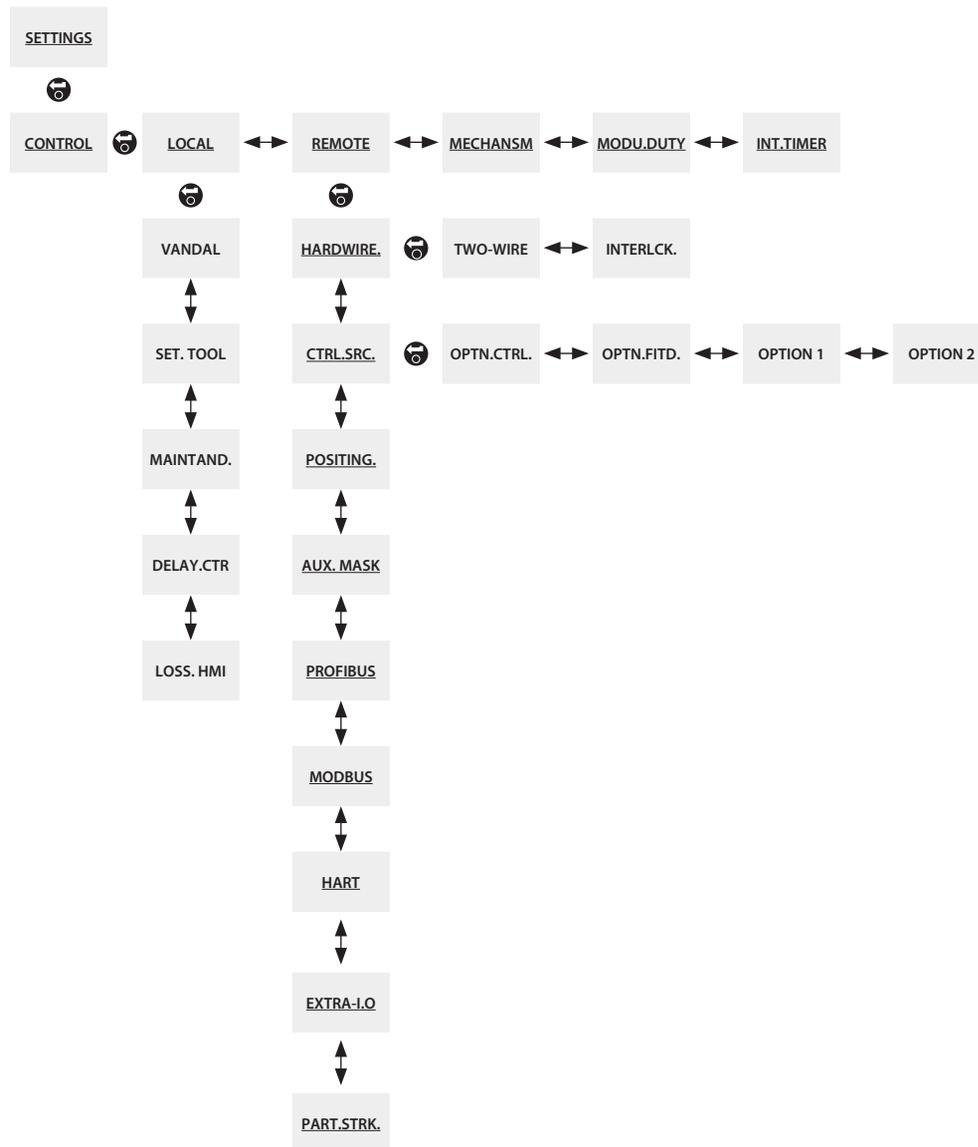
The above menu map should be used as a navigation prompt to improve configuration efficiency. An underlined text string indicates a menu. A standard text string indicates a setting.
