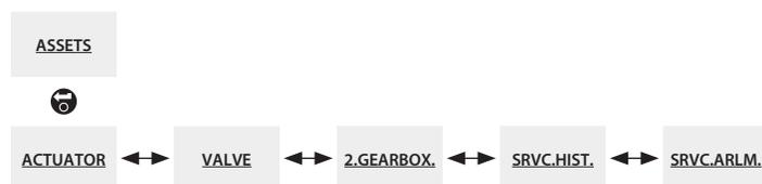
The above menu map should be used as a navigation prompt to improve configuration efficiency. An underlined text string indicates a menu. A standard text string indicates a setting.
