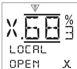
**Open [OPEN]:** - Displays the current Local Open signal status. When active, this indicates the local controls have been turned to open and a local control open signal is being received.
