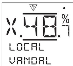
**Vandal [VANDAL]:** - To prevent unauthorised changes to the actuator operating mode, vandal resist can be enabled to restrict operation to one specific mode ignoring the position of the local selector knobs.
