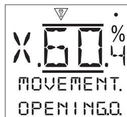
**Opening [OPENING]:** - Displays the actuator Moving Open status. When active, this status indicates that the actuator is moving open.
