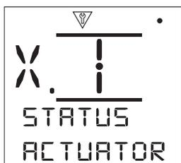
This menu displays the actuator switch statuses. The checkbox indicates that the condition is present.
