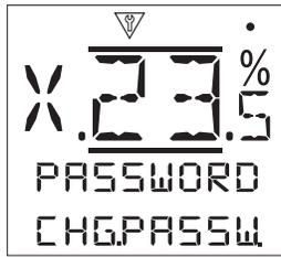
**Change PW [CHANGE.PW.]:** - This feature allows the user level password to be changed from the default ROTORK. Protection from unauthorised access is vital to maintaining site security and process control integrity.
