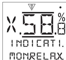
**Monitor Relay [MON.RELA.]:** - Displays the Monitor Relay status. A checked checkbox shows the relay is active, whilst an unchecked checkbox represents inactive.
