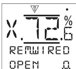
**Open [OPEN]:** - Displays the current Remote Hardwired Open signal status. When active, this indicates that an open signal is being received from the remote hardwired control.
