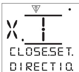
**Direction to Close [DIRECTIO.]:** - Specify the direction of operation required to close the valve - Clockwise or Anti-Clockwise.
