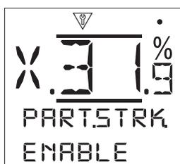
**Enable [ENABLE]:** - Specify whether the partial stroke function is enabled or disabled.
