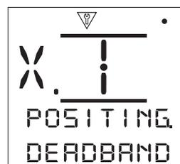
**Deadband [DEADBAND]:** - Affects positioning accuracy as a response to the process control system desired value (DV) signal position. A smaller deadband increases accuracy, however the widest deadband should be set whilst maintaining good control in order to protect the mechanical valve from excessive wear and/or to keep the actuator within its electrical rating.
