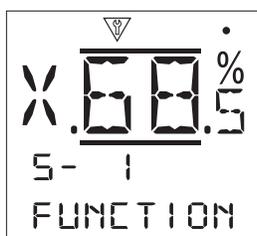
**S Function [FUNCTION]:** - The available contact functions that can be configured for S contact relays are detailed in table 1 opposite.
