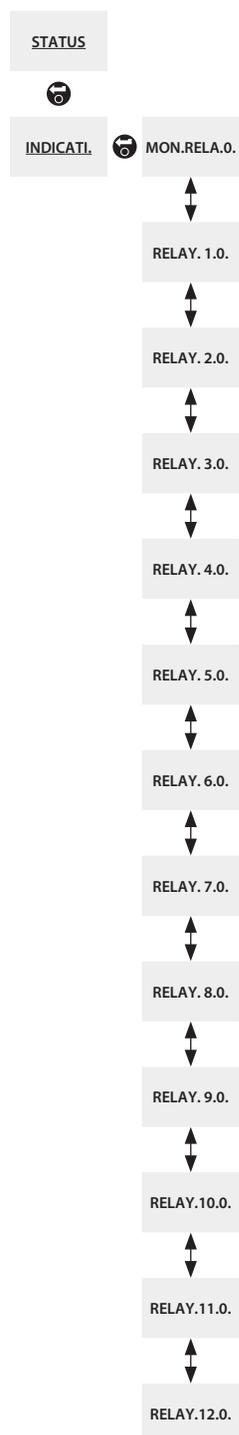
The above menu map should be used as a navigation prompt to improve configuration efficiency. An underlined text string indicates a menu. A standard text string indicates a setting.
