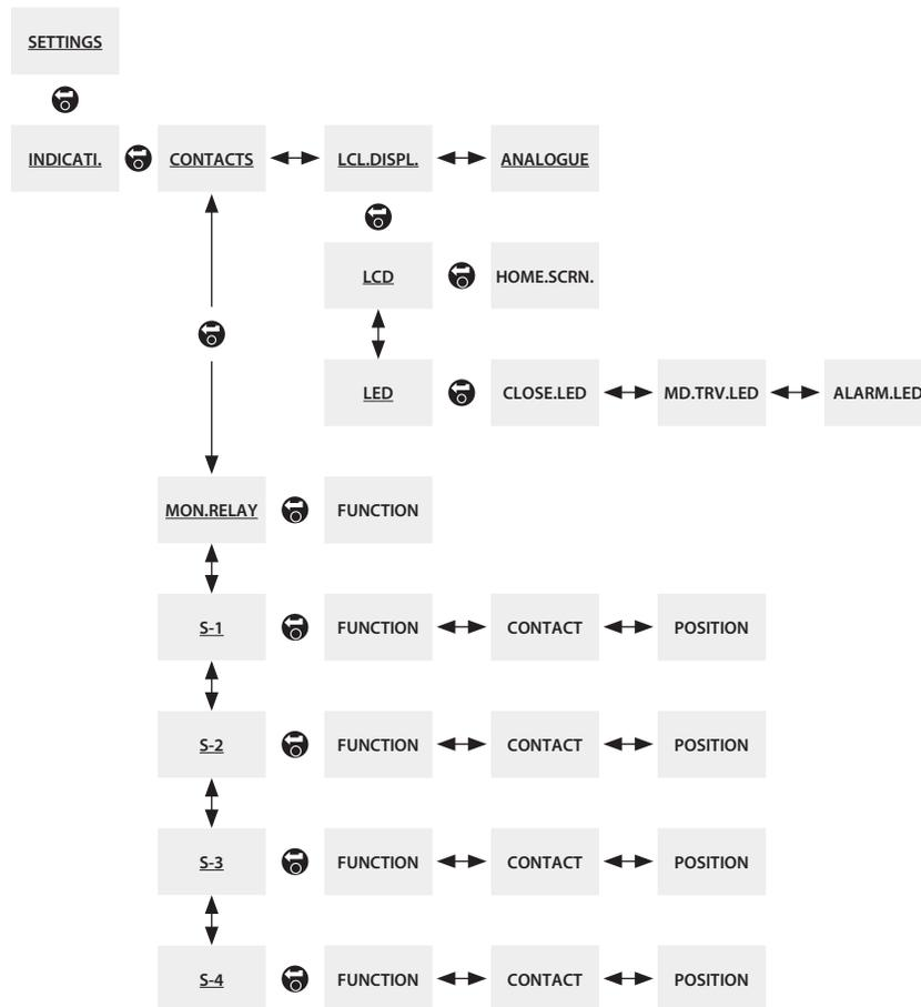
The above menu map should be used as a navigation prompt to improve configuration efficiency. An underlined text string indicates a menu. A standard text string indicates a setting.
