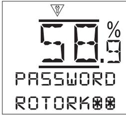
The Centronik control module offers password protection that prevents modification to any configuration settings by unauthorised operators.
