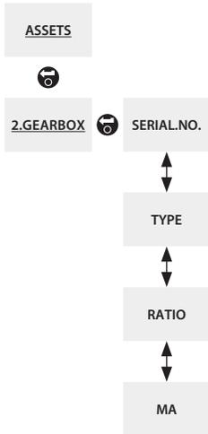
The above menu map should be used as a navigation prompt to improve configuration efficiency. An underlined text string indicates a menu. A standard text string indicates a setting.
