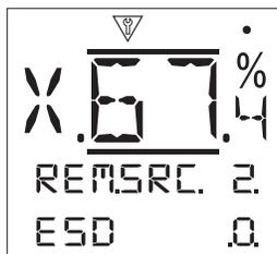
**ESD [ESD]:** - Displays the current Remote Source 2 ESD signal status. When active, this indicates that an ESD (Emergency Shut Down) signal is being received from remote source 2.
