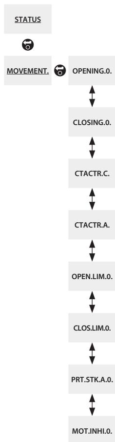
The above menu map should be used as a navigation prompt to improve configuration efficiency. An underlined text string indicates a menu. A standard text string indicates a setting.
