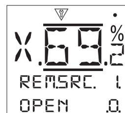
**Open [OPEN]:** - Displays the current Remote Source 1 Open signal status. When active, this indicates that an open signal is being received from remote source 1.
