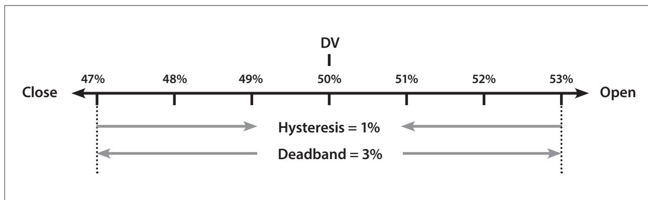
**Example:** An actuator set with a 3% deadband and a 1% hysteresis and a control system new Desired Value (DV) of 50% will come to rest between 48% and 53% when moving from a position less than 47%, and between 52% and 47% when moving from a position greater than 53%.
