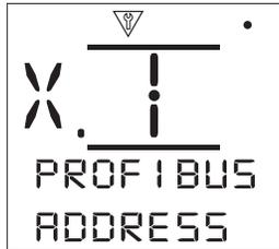
**Address [ADDRESS]:** - The Profibus module must be allocated a unique address in the Profibus system. Changes made to the address will take effect immediately. The range of address is 1 – 126. If flying redundancy is being used in a dual channel system then the range of address is 1 – 62.
