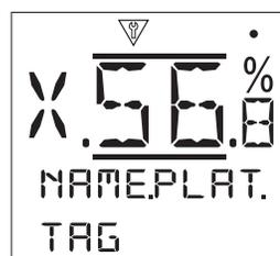
**Tag [TAG]:** - The tag entry will be shown on the actuators set home screen display. The tag name entered should be the valve and/or actuator reference that identifies the asset within the site process control scheme. If the tag was supplied at time of order, Centork will populate the entry automatically.
