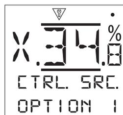
This menu shows common actuator response settings for all CK option cards during a loss of signal condition.
