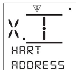
**Address [ADDRESS]:** - The HART option must be allocated a unique address in the HART system. Changes made to the address will take effect immediately. The range of address is 0 - 63.
