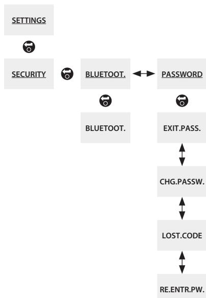
The above menu map should be used as a navigation prompt to improve configuration efficiency. An underlined text string indicates a menu. A standard text string indicates a setting.
