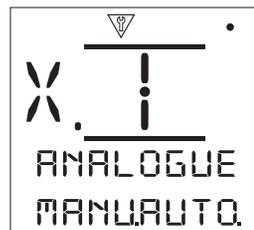
**Manual Auto [MANU.AUTO.]:** - Enable or disable the manual auto switch that determines control between analogue and hardwired inputs.
