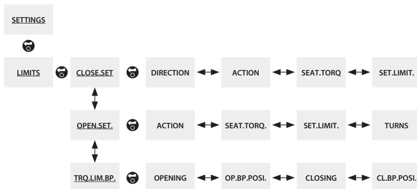
The above menu map should be used as a navigation prompt to improve configuration efficiency. An underlined text string indicates a menu. A standard text string indicates a setting.
