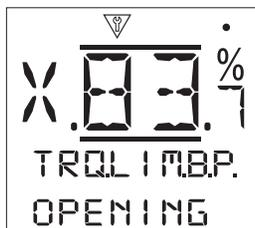
**Opening [OPENING]:** - Turn the Torque Limit Bypass on or off in the open direction.
