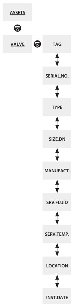
The above menu map should be used as a navigation prompt to improve configuration efficiency. An underlined text string indicates a menu. A standard text string indicates a setting.
