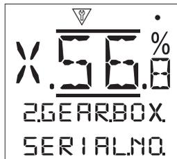
**Serial No [SERIAL.NO.]:** - Displays the serial number of the gearbox.
