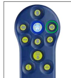
\* Hold selector position for 3 seconds to special input function.
