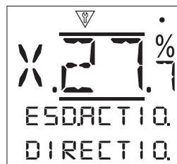
**Direction [DIRECTIO.]:** - Set the desired ESD movement direction.
