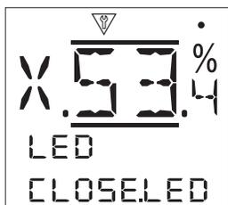
**Close LED [CLOSE.LED]:** - Specify the colour of the close limit indication LED on the local display – Green or Red (the Open limit will return the opposite colour to distinguish between each position). .
