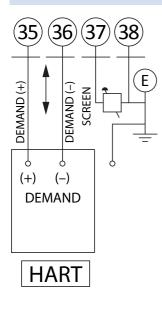
Network connections are made to the terminals of the actuator as defined in the wiring diagram. Shown here is a typical arrangement used in standard wiring diagrams, in this case HART connections here are made to terminals 35 (+) and 36 (-) of the terminal bung. The wiring diagram should be checked to confirm the correct terminal numbers and to confirm which terminal has positive and which terminal has negative polarity.
