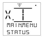
Status screens on the CK Centronik module are designed to provide diagnostic assistance. The displayed information is live data taken from the main control processor and can be used to view control signals, alarms, movement and internal diagnostic data.
