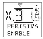
**Enable [ENABLE]:** - Specify whether the partial stroke function is enabled or disabled. **To O To S**.
