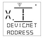
**Address [ADDRESS]:** - The DeviceNet option must be allocated a unique address in the system. Changes made to the address will take effect immediately. The range of address is 0 to 63.
