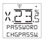
**Change PW [CHANGE.PW.]:** - This feature allows the user level password to be changed from the default ROTORK. Protection from unauthorised access is vital to maintaining site security and process control integrity.
