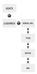
The above menu map should be used as a navigation prompt to improve configuration efficiency. An underlined text string indicates a menu. A standard text string indicates a setting.
