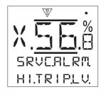
Close Hi Alarm % [CL.HI.TP.LV.]: - Allows the user to set a value for an open torque alarm. E.g. 70%. 6
