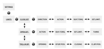
The above menu map should be used as a navigation prompt to improve configuration efficiency. An underlined text string indicates a menu. A standard text string indicates a setting.
