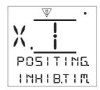
**Inhibit Time [INHIB.TIM.]:** - Sets a delay after the actuator stops as a result of reaching a position consistent with a new DV position. For the period set, the actuator will not respond to a change in DV. Inhibit time is used to prevent unwanted operation as a result of a rapidly oscillating or fluctuating DV signal or to slow actuator response in order to protect the mechanical valve from excessive wear and/or maintain actuator within its electrical rating.
