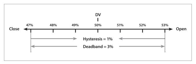
**Example:** An actuator set with a 3% deadband and a 1% hysteresis and a control system new Desired Value (DV) of 50% will come to rest between 48% and 53% when moving from a position less than 47%, and between 52% and 47% when moving from a position greater than 53%.
