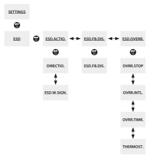
The above menu map should be used as a navigation prompt to improve configuration efficiency. An underlined text string indicates a menu. A standard text string indicates a setting.
