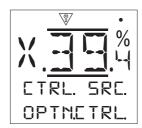
Set the control sources and control priorities for the actuator during normal operation.
