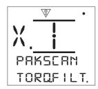
**Torque Filter [TORQ.FILT.]:** - Set to enable or disable auto reporting of the historical torque logs.
