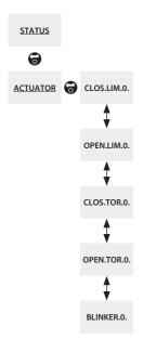
The above menu map should be used as a navigation prompt to improve configuration efficiency. An underlined text string indicates a menu. A standard text string indicates a setting.
