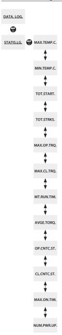
The above menu map should be used as a navigation prompt to improve configuration efficiency. An underlined text string indicates a menu. A standard text string indicates a setting
