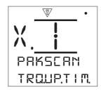
**Torque Update Time [TRQ.UP.TIM]:** - Torque update time (minutes) value is refreshed from a stationary actuator. If torque data is not required then the update time should be disabled. Range 5 to 255 minutes. Less than 5 will disable this feature.
