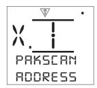
**Address [ADDRESS]:** - The Pakscan Field Control Unit option must be allocated a unique loop node address. Changes made to the address will take effect immediately. The range of address is 1 to 240.
