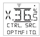
Factory set for the control options fitted. Up to 2 options can be fitted and will be indicated in this menu. Unused allocations will be set to Disabled.
