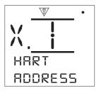
**Address [ADDRESS]:** - The HART option must be allocated a unique address in the HART system. Changes made to the address will take effect immediately. The range of address is 0 - 63.
