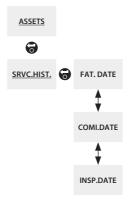
The above menu map should be used as a navigation prompt to improve configuration efficiency. An underlined text string indicates a menu. A standard text string indicates a setting.
