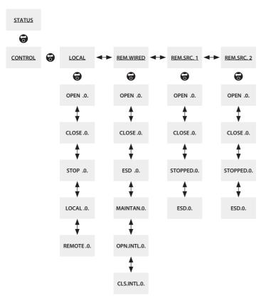
The above menu map should be used as a navigation prompt to improve configuration efficiency. An underlined text string indicates a menu.
